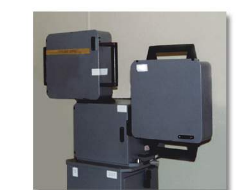
IUS film recorders comprised of Scitairre Cine III CRT and MSM 65mm 15-perf camera.
